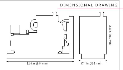
NL673L4 Overall Dimensions L x W x H: 32.8 x 17.1 x 26.8 inch (834 x 435 x 650 mm) Dimensions given in inches (mm). Dimensions subject to change without notice. Contact dealer or visit www.northern-lights.com for most current installation drawings.
